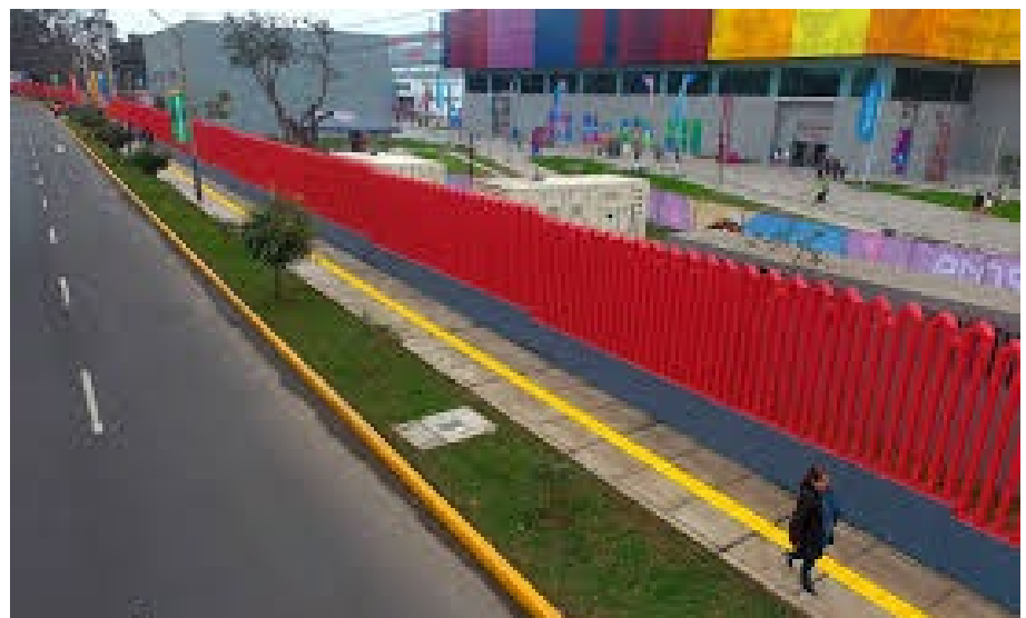
Yellow strip with bump dots on city streets that help guide blind or visually impaired individuals.
